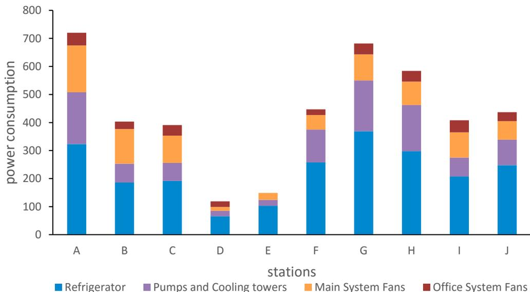
Fig.2 Subentry instantaneous power consumption statistics
