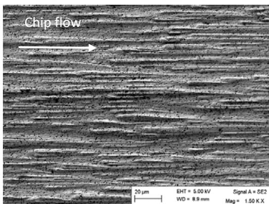
**Figure 1.** Wear characteristics of worn cemented carbide within the crater on the insert rake face. Note the formation of ridges parallel with the chip flow direction. Cutting time 12 seconds.
