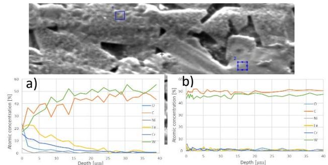
**Figure 3.** AES depth profiles showing the element composition of the two types of WC grain surface morphologies found in the crater region. Cutting data;  $v_c$ : 240 m/min, cutting time 12 seconds.
