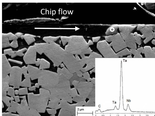
**Figure 2.** Cross section cemented carbide after 12 seconds turning at cutting speed of 240 mm/min and feed rate of 0.2 mm/rev.
