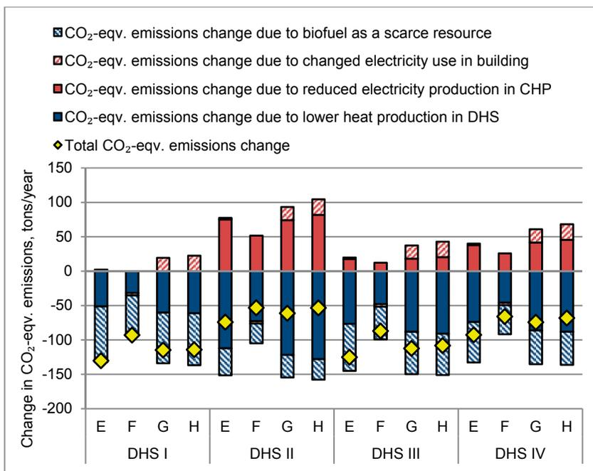
Figure 9. The CO<sub>2</sub>-eqv. emissions from each refurbishment package in each district heating system divided into sources of origin.
