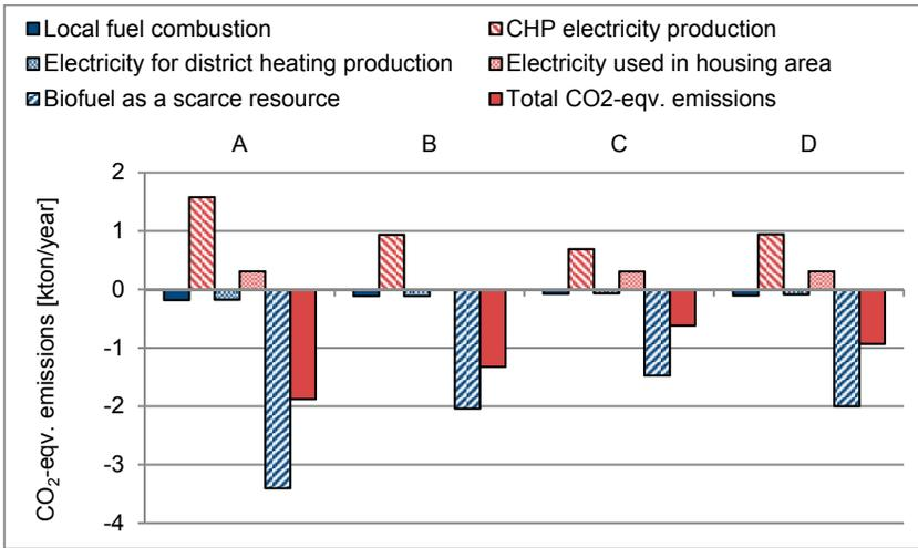
Figure 7. The total CO<sub>2</sub>-eqv. emissions for each refurbishment package is the sum of CO<sub>2</sub>-eqv. emissions from different sources in the energy system.
