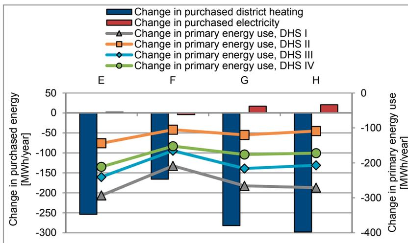
Figure 10. The changes in purchased district heating and electricity for each refurbishment package compared to the changes in primary energy use for each refurbishment package in each district heating system.
