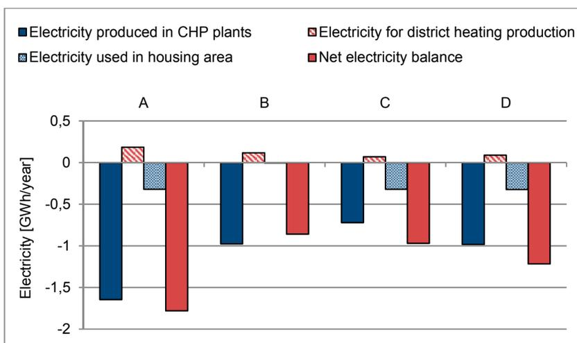
Figure 6. The net electricity balance is defined as the sum of the changes of the electricity produced in CHP plants, the electricity used for district heating production and the electricity used in the housing area.
