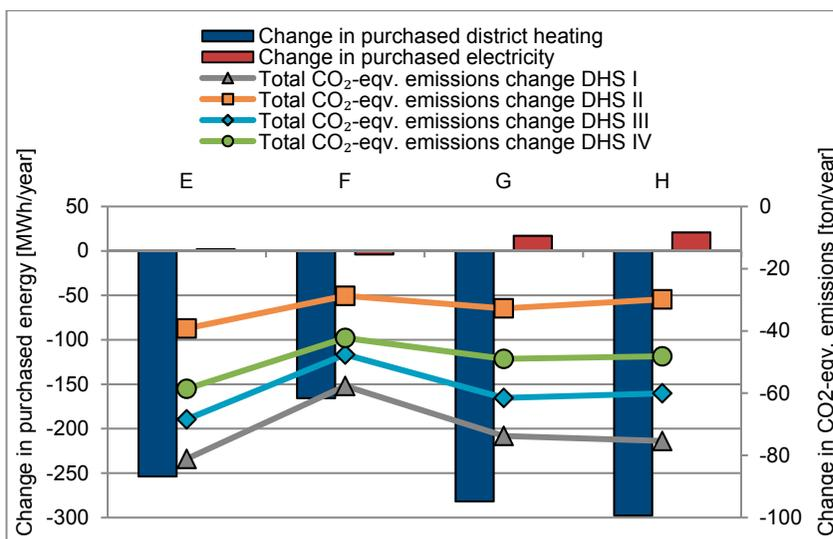
Figure 8. The changes in purchased district heating and electricity for each refurbishment package compared to the changes in CO<sub>2</sub>-eqv. emissions for each refurbishment package in each district heating system.
