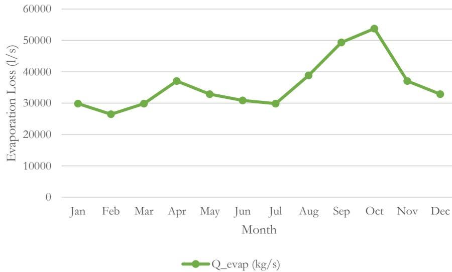
Figure 2.7 Evaporation rate for KGUPS dam calculated for the year 2018
