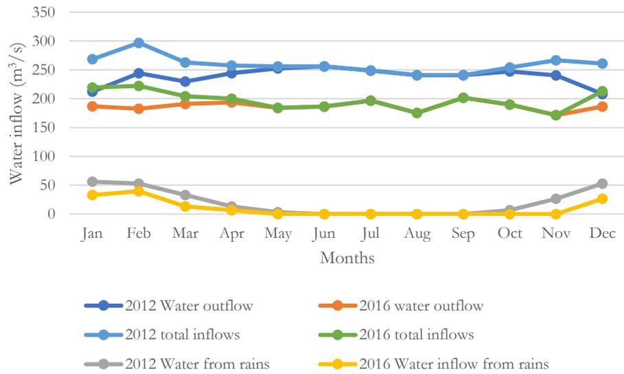
Figure 2.6 Water outflow and inflows into the KGUPS dam for 2012 and 2016
