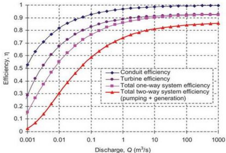
Figure 2.10 Efficiency and flowrate of the typical Francis turbine-pump system [26]
