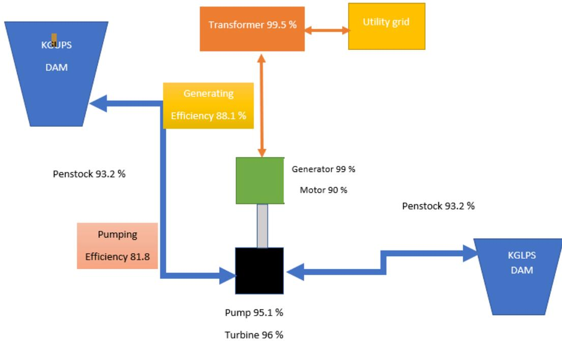
Figure 2.9 Losses breakdown of the pumping scheme
