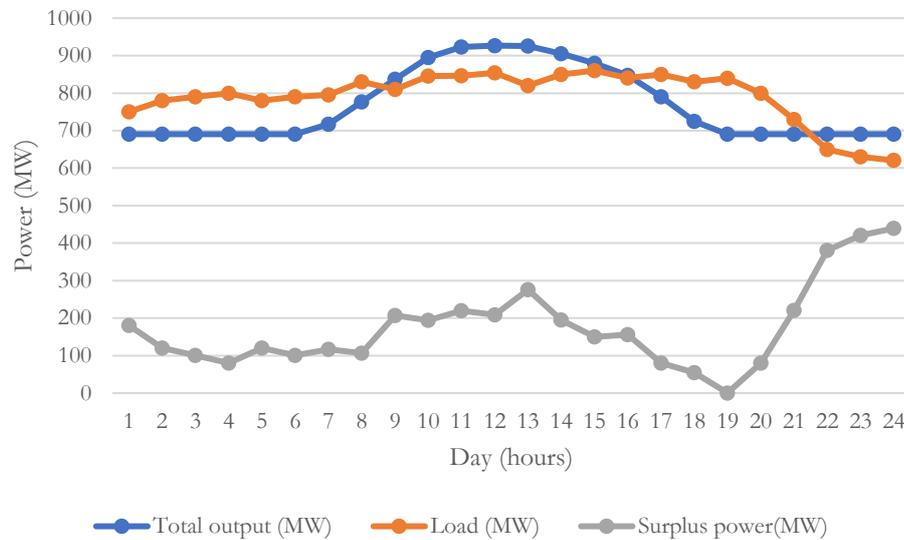
Figure 3.5 Scenario five for 20<sup>th</sup> October 2012 for KGUPS with PHES and PV system
