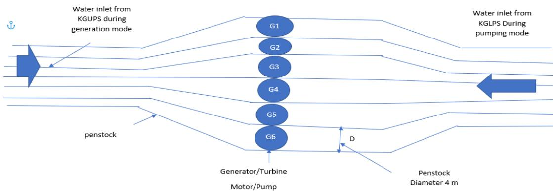
Figure 2.8 Schematic arrangement of penstocks and machines
