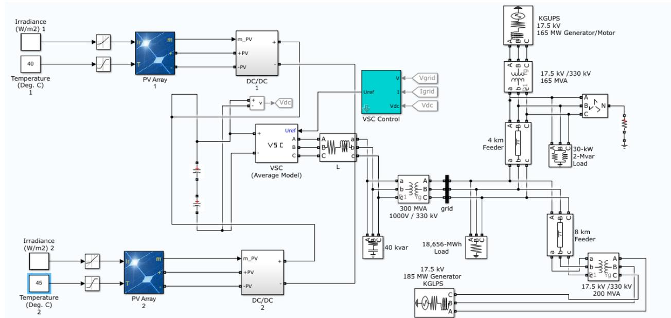
Figure 2.11 proposed system model screen excerpt from MATLAB Simulink
