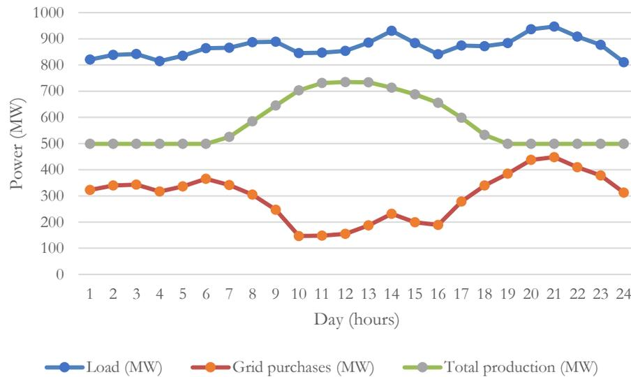
Figure 3.3 Performance of KGUPS with PHES and PV for October 20<sup>th</sup>, 2016 (Dry period)
