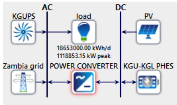
Figure 2.12 System model from Homer software
