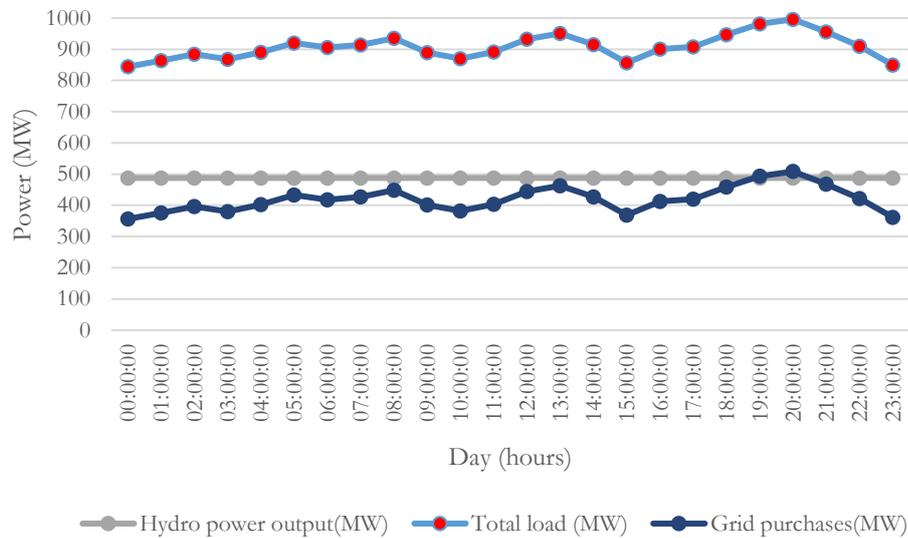
Figure 3.1 Simulation results for the year 2016 with no PV and PHES systems
