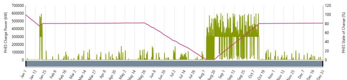
Figure 3.6 State of charge and charge power of the PHES system for the year 2012
