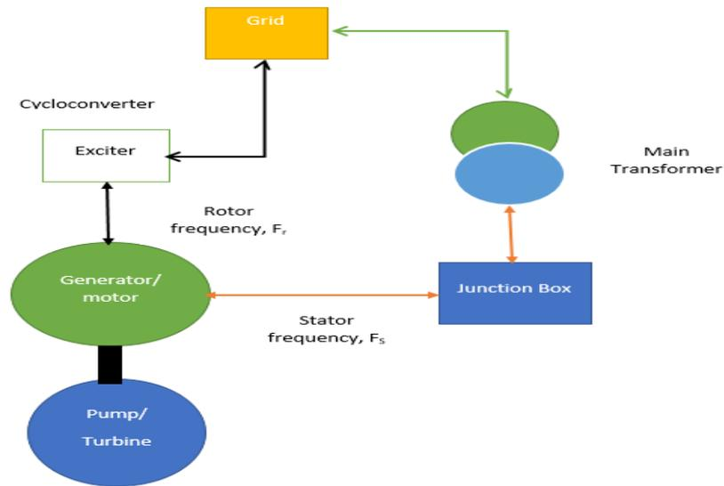
Figure 1.8 Double fed induction machine adjustable speed control [17]
