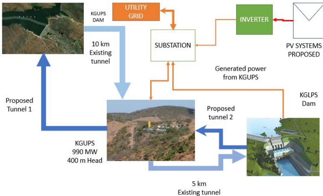
Figure 1.3 Existing and proposed system layout
