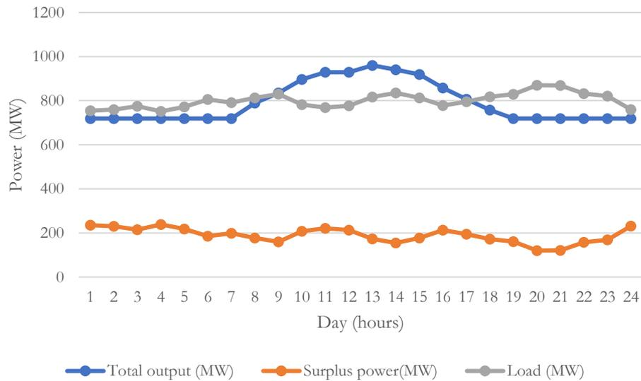
Figure 3.4 KGUPS performance with PV and PHEs system for the year 2012 on 15<sup>th</sup> June
