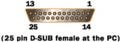
Fig. 1.1 DB-25 connector (Courtesy of HowStuffWorks Inc.)
