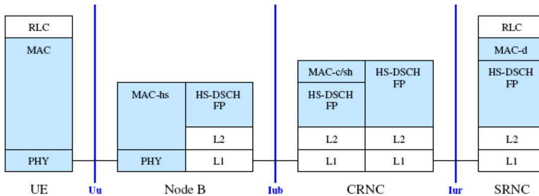
Figure 2 HSDPA protocol architecture, modified parts highlighted
