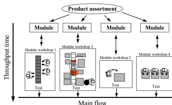
Figure 1: Parallel activities in the module assembly [Erixon 1998].
