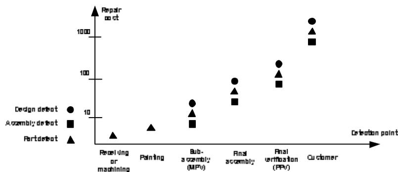
Figure 2: Repair cost as a function of defect and detection point, schematically.
