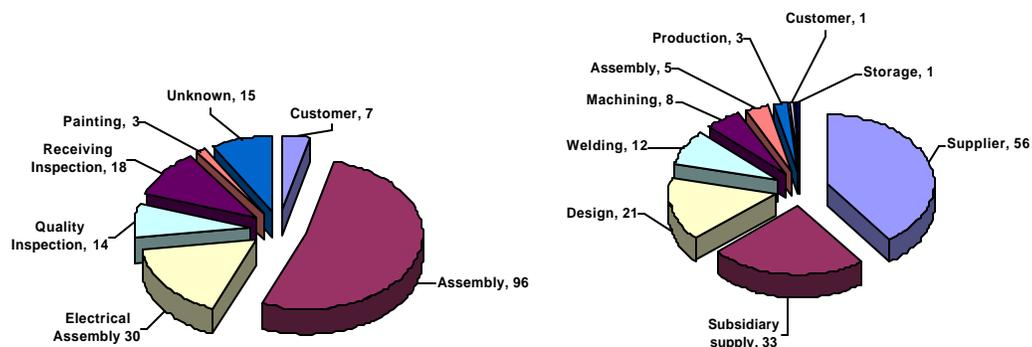
Figure 1: (Left) point of detection of 183 defects in 150 units, defect rate 1.22 during one produced order, (right) 140 known defect causes of 183 defects in 150 units at company B.
