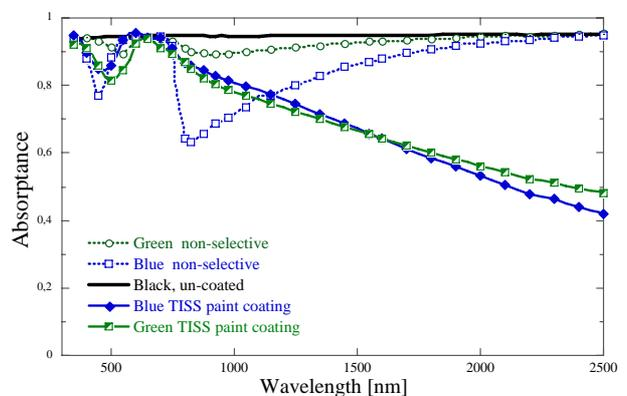
Fig. 2. Absorptance of the un-coated black absorber, of the absorber coated with green/ blue TISS paints and with non-selective green/blue paints.
