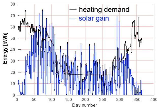
Fig. 7. Solar combisystem with façade collectors: Total heating demand and solar gain of a well-insulated single-family house for Oslo climate, calculated with the simulation program SolDat.
