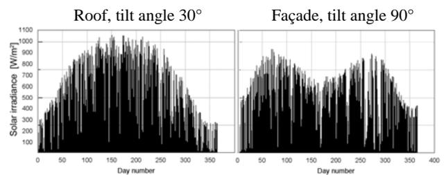
Fig. 5. Solar irradiance per square meter on a roof with 30° tilt angle and on the façade (90° tilt angle) calculated with the simulation program SolDat for the location Oslo (latitude 60°).
