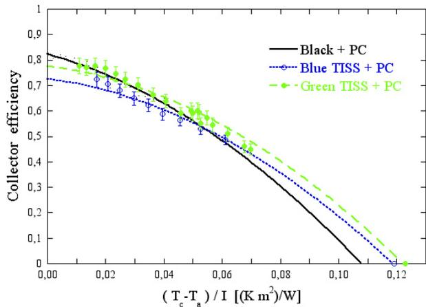
Fig. 4. Measured collector efficiency of the polymeric absorber painted with blue and green TISS paints and with 10 mm polycarbonate twin-wall sheet as collector cover.
