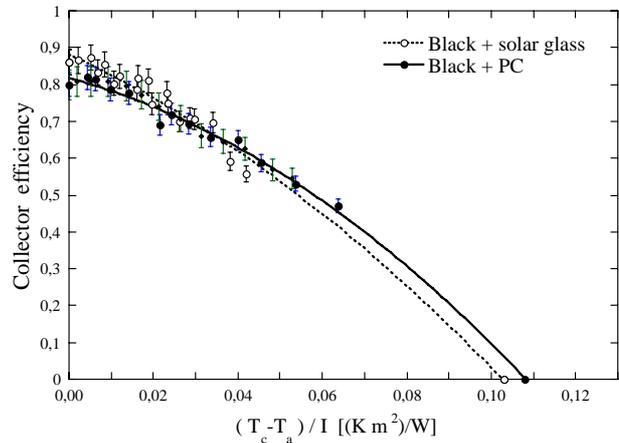
Fig. 3. Measured collector efficiency of the black, uncoated polymeric absorber with two different collector covers: 10 mm polycarbonate twin-wall sheet and 4 mm solar glass.
