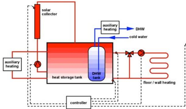
Fig. 1. Hydraulic scheme of a solar heating system with drain-back design and polymeric façade collectors.
