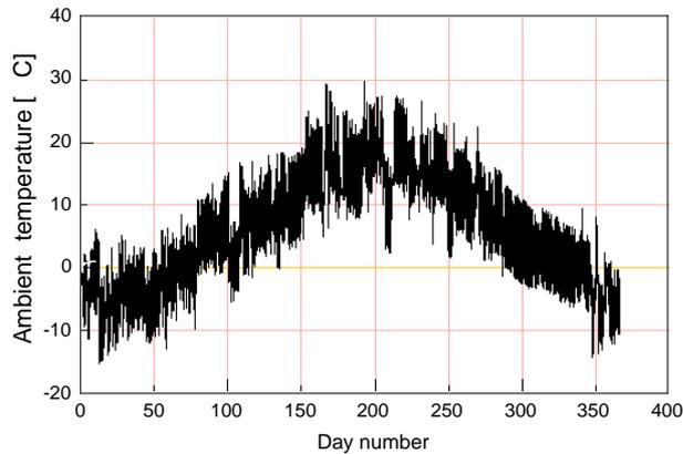
Fig. 6. Ambient temperature for Oslo climate (Norway, latitude 60°), calculated with the simulation program SolDat.
