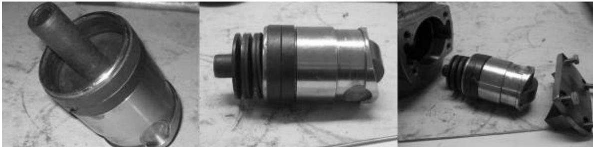
Figure 8: Left: the piston and the guiding tube which the disc spring are inserted onto. Centre: the disc spring needs to be in 12 pairs of discs on the pistons. Right: Finally, the pistons with the springs are inserted into the cylinder from two opposing directions.
