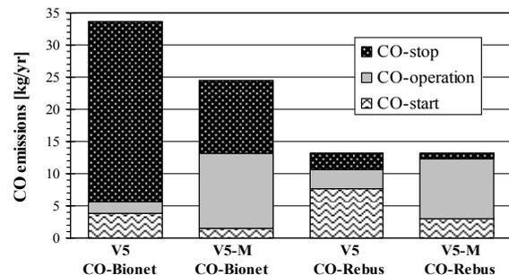
**Figure 5:** Comparison of annual CO-emissions for the ON-OFF control (V5) and the modulating power control (V5-M) for the boiler used in the study (Bionet) and for the same boiler with other CO-emission factors (Rebus). Rebus has slightly higher emissions during operation and start (4.4 g) but lower stop emissions (1.4 g) [17].
