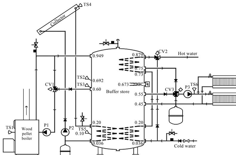
Figure 2: The simulated solar combisystem with connection heights on the store.
