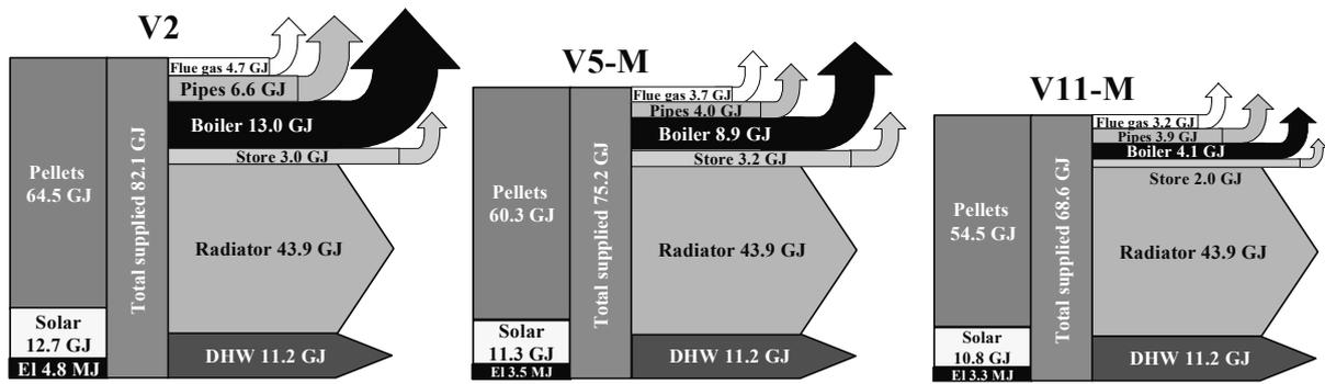
**Figure 3:** The simulated energy balance in the systems V2, V5-M and V11-M from Table I.
