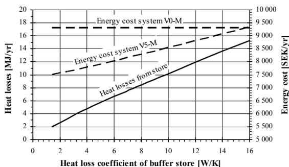
**Figure 4:** Annual heat losses from store and energy costs as a function of the heat loss coefficient of the store for system V5-M. According to [1]  $UA \approx 6$  W/K corresponds to 100 mm mineral wool + air tight cover + pipe connections straight through insulation.  $UA \approx 2.6$  W/K corresponds to 150 mm rubber foam + air tight cover + pipe connections under insulation down to the floor.
