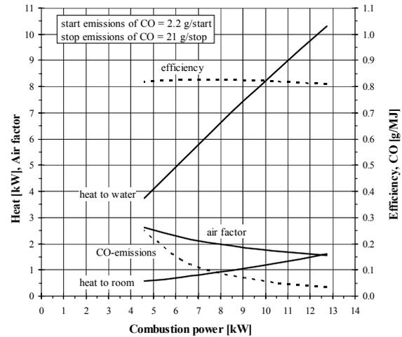
Figure 1: The characteristic of the simulated boiler [17].
