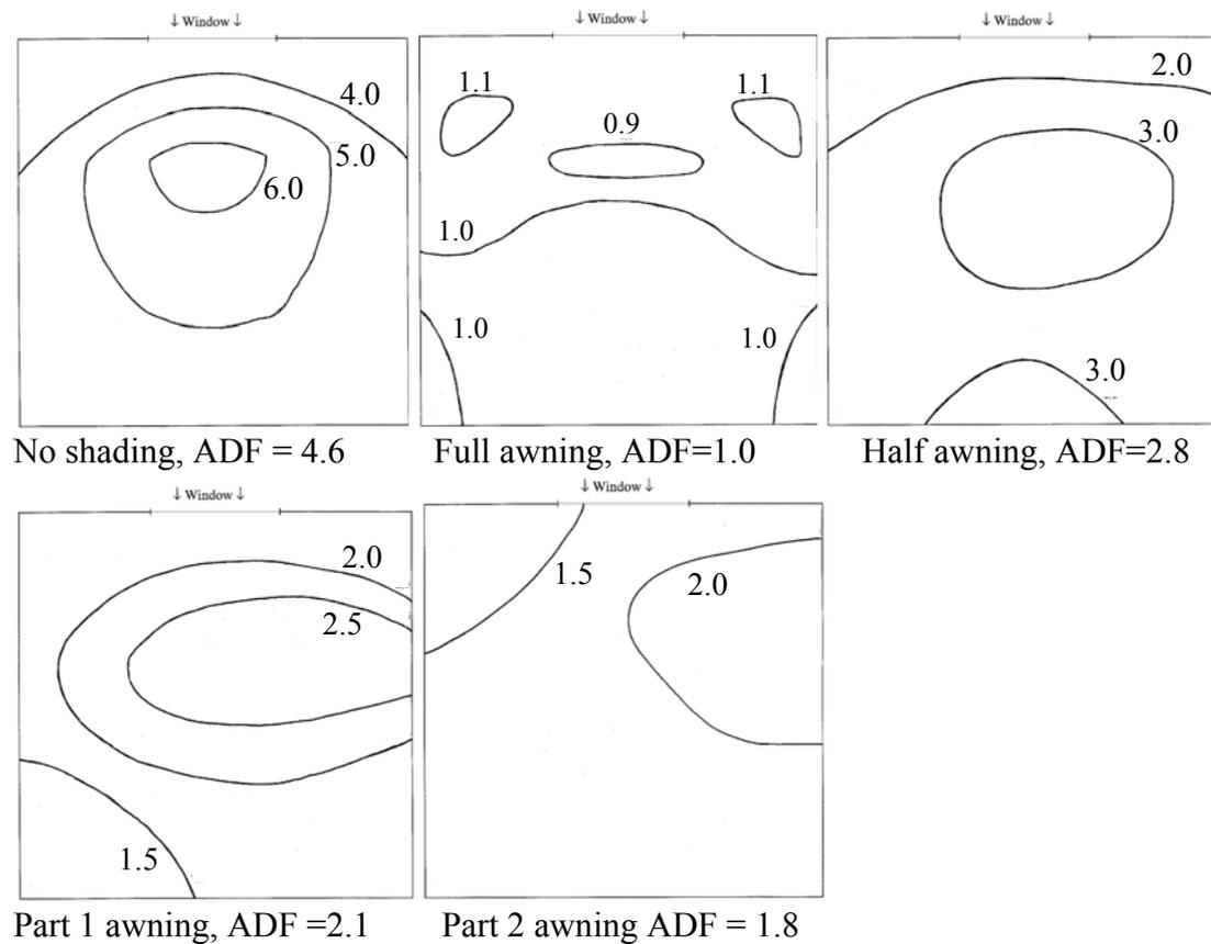
Figure 4. Contour maps of the daylight factor at the bottom of the box, using different geometries of the awning (see table 1). A window without awning is shown as reference.
