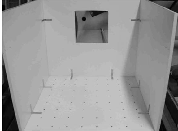
Figure 2. Picture of the scale model before the roof and back side was mounted. The window hole is seen from inside.
