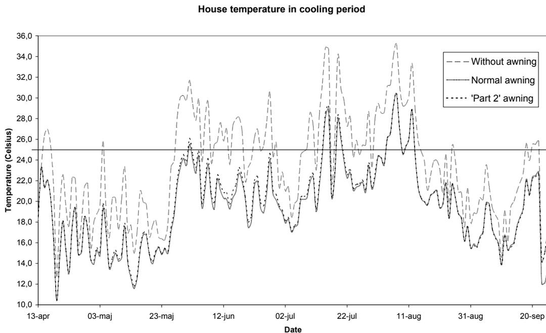
Fig. 5. Mean indoor temperature with no awnings, normal awnings and part 2 awnings.
