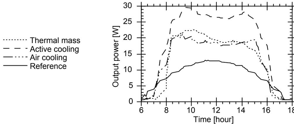
Figure 3. Example of output for some different concentrator modules during a clear day. Data from August 11, 1998.
