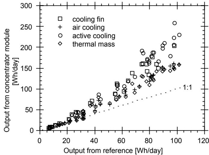
**Figure 2.** Input/output diagram showing the daily output from the concentrator modules vs. the output from the reference module. All measurement days are included in the diagram.
