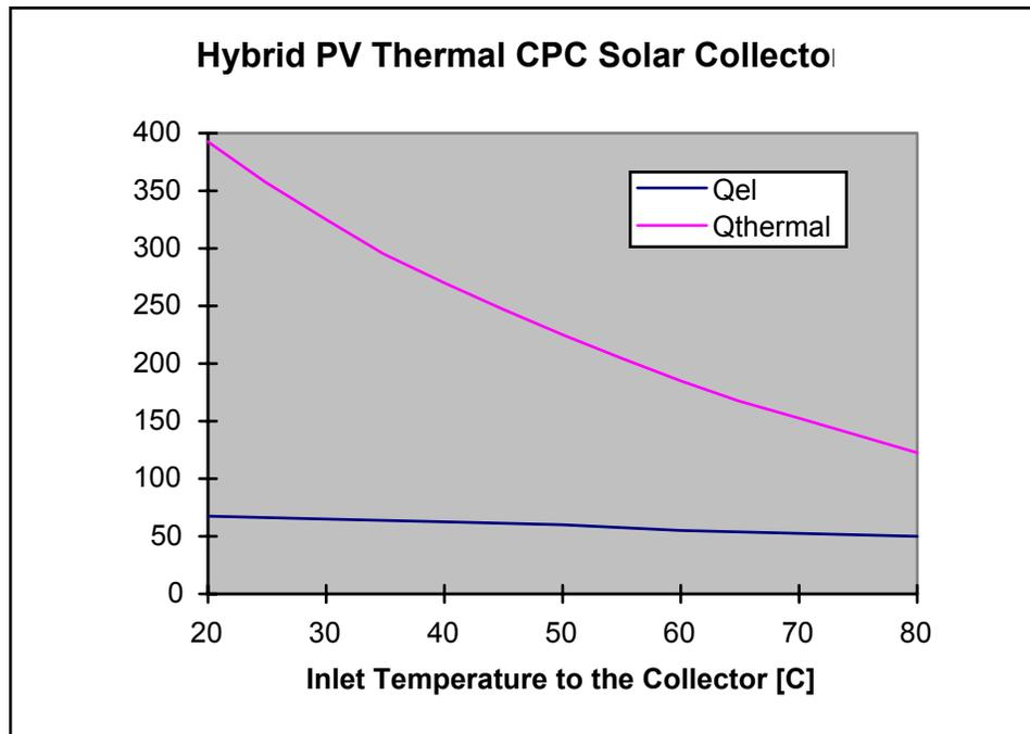
Figure 4. Expected output from a Hybrid PV/thermal solar collector. Collector parameters are defined in the text. Climatic data from Stockholm, lat. 59.4°N.
