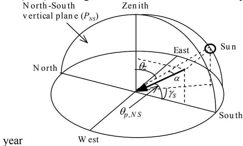
Figure 1. Definition of the south projection angle  $\theta_{p,NS}$ , which is the angle between the projection of the sun position vector on to a north-south vertical plane and the south horizon.  $\theta_z$  = solar zenith angle;  $\gamma_s$  = solar azimuth angle.
