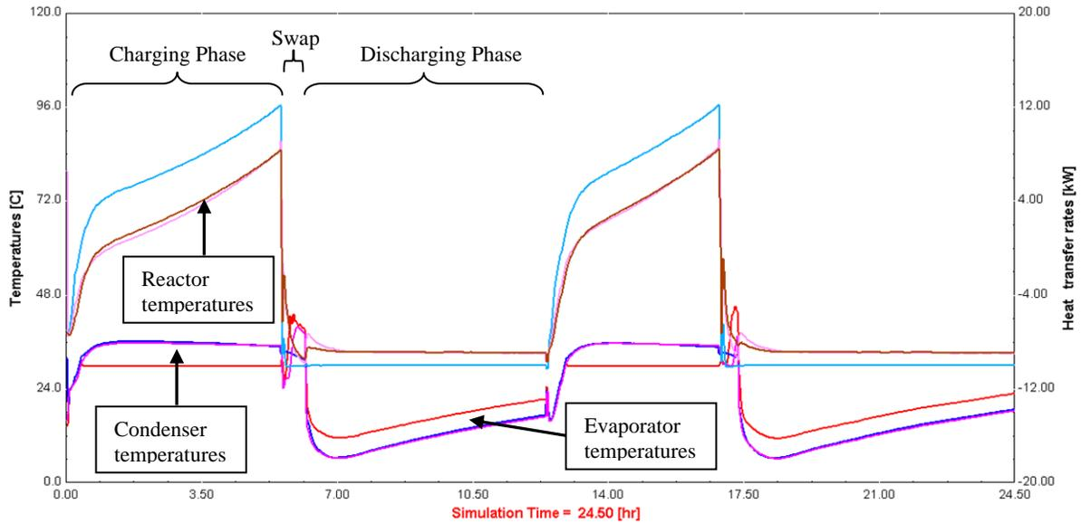
Figure 3b: Measured and simulated inlet/outlet temperatures to reactor and condenser/evaporator heat exchangers.
