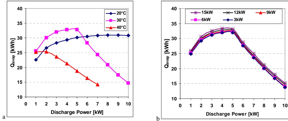
Figure 5: Variation of the cold storage capacity ( $Q_{evap}$ ) with the discharge and charge powers as well as cooled water temperatures.
