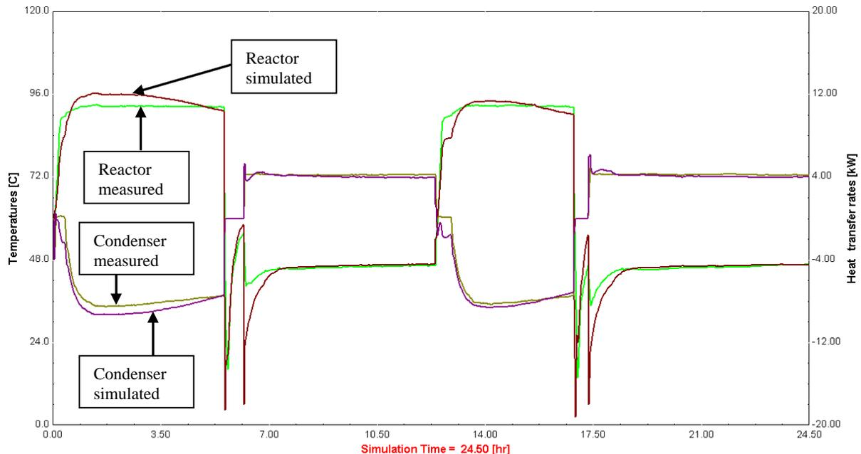
Figure 3a: Measured and simulated heat transfer rates for reactor and condenser for two full cycles of a single unit.
