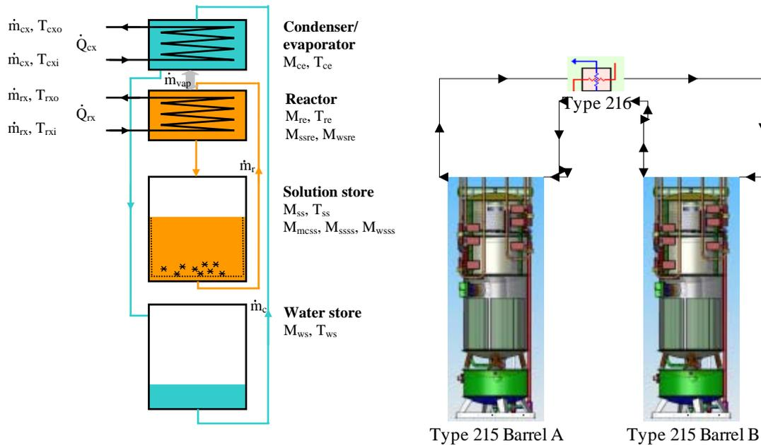
Figure 1: Schematic of Type 215 single TCA unit model (left) and a complete TCA machine in TRNSYS studio (right), comprising two units (Type 215) and a switching/controller unit (Type 216).
