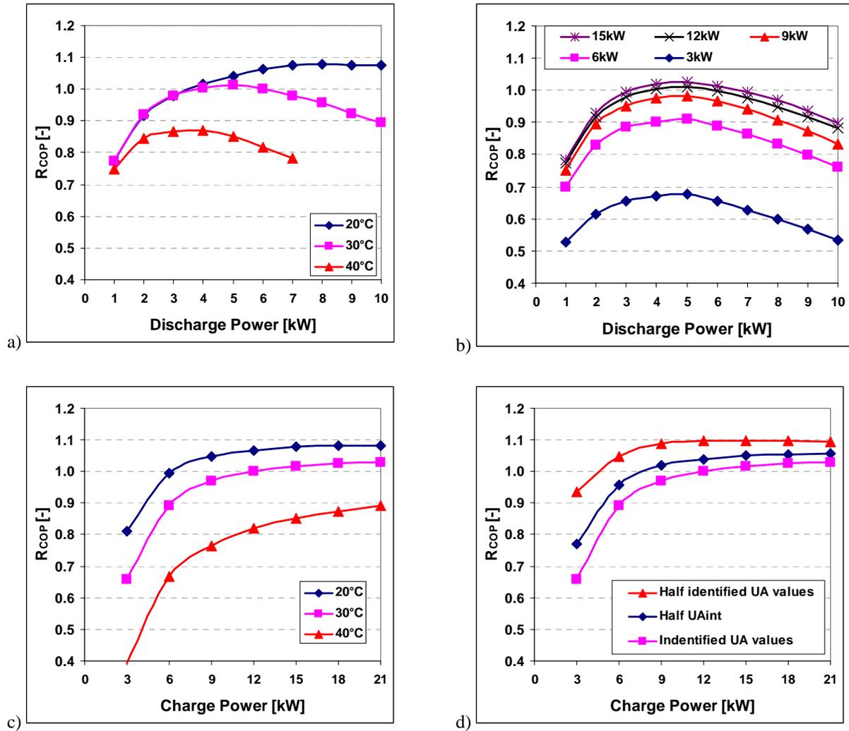
Figure 4: Normalised COP values ( $R_{COP}$ ) versus discharge powers at different cooling water temperatures (a) and charge powers (b): versus charge power at different cooling water temperatures (c) and heat loss coefficients (d).
