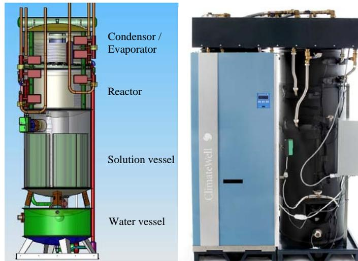
Figure 1: Schematic of a single TCA unit (left) and the complete commercial CW10 machine (right), comprising two barrels (units) and a switching unit above.
