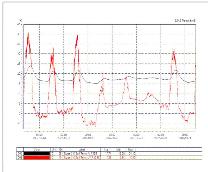
Figure. 9 – The temperatures on the interior and exterior surfaces of the south facing roof on cabin C are given for the late October 2007- test period.
