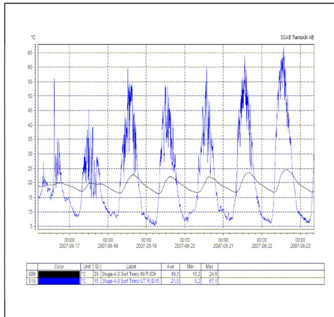
Figure. 3 – The temperatures on the interior and exterior surfaces of the south facing roof on cabin A are given for the late August 2007- test period.
