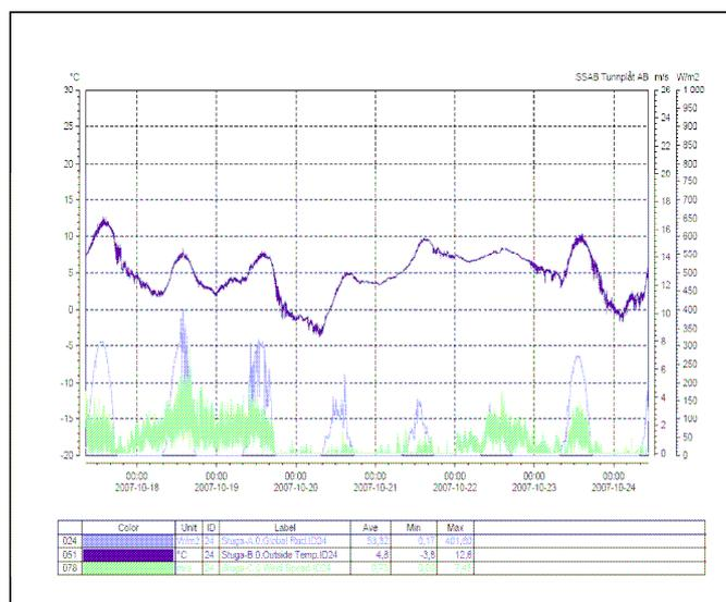
Figure. 6 – The global solar radiation, the outside air temperature and the wind speed close to the roof top are given as functions of time for a 7 days period in late October 2007.
