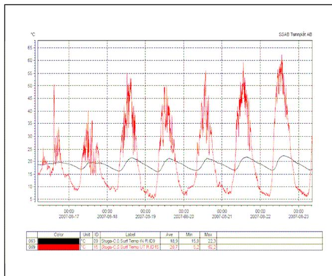
Figure. 4 – The temperatures on the interior and exterior surfaces of the south facing roof on cabin C are given for the late August 2007- test period.
