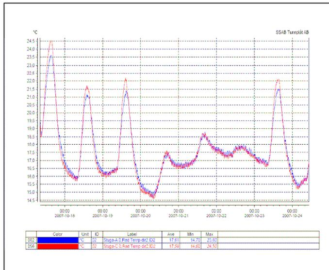
Figure. 7 – The radiation temperatures measured by pyrometers facing the upper part of the cabin interior in cabins A and C during late October 2007.
