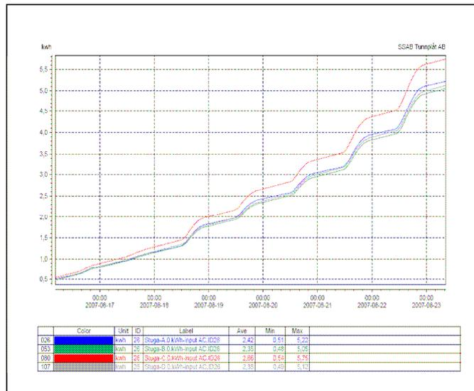
Figure. 5 – The accumulative energy used by the air-conditioning units in cabins A, B, C and D during late August 2007.
