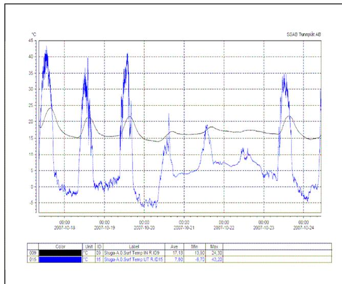
Figure. 8 – The temperatures on the interior and exterior surfaces of the south facing roof on cabin A are given for the late October 2007- test period.
