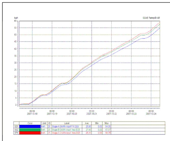
Figure. 10 – The accumulated energy used for heating in cabins A, B and C is given for the late October test period.
