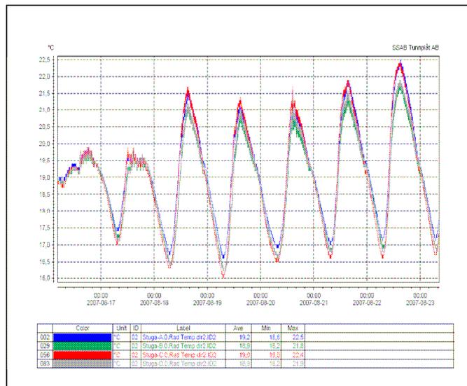
Figure. 2 – The radiation temperatures measured by pyrometers facing the upper part of the cabin interior in cabins A, B, C and D during late August 2007.
