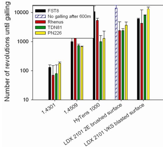
**Figure 4. Gallings resistance for the different stainless steel grades and lubricants after lubricated sliding contact with Vancron 40.**
