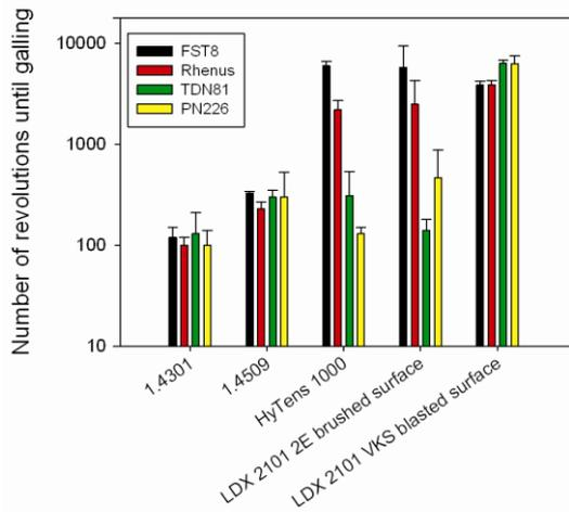
**Figure 3. Gallings resistance for the different stainless steel grades and lubricants after lubricated sliding contact with Vanadis 10**
