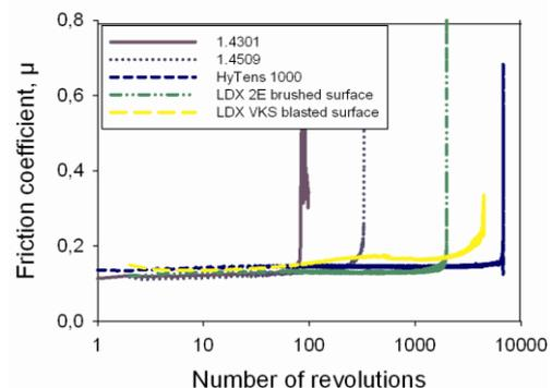
**Figure 2. Friction characteristics of the stainless steel grades in lubricated sliding contact with Vanadis 10 using FST 8 as lubricant.**
