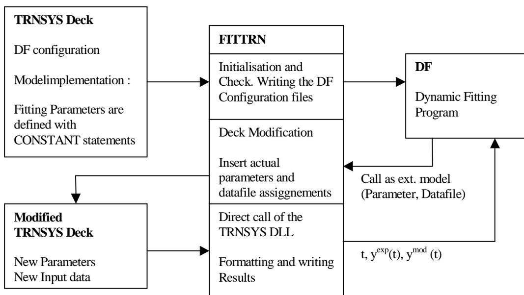
Figure 2. Communication between the programs Trnsys, DF and Fittrn. Figure taken from Fittrn manual, courtesy of SPF, Rapperswil.
