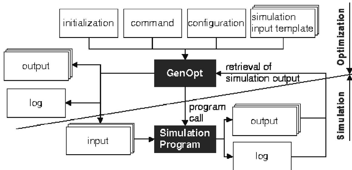
Figure 4. Interface between GenOpt and the simulation program (From GenOpt Manual, courtesy of LBNL, Berkeley Univ.).
