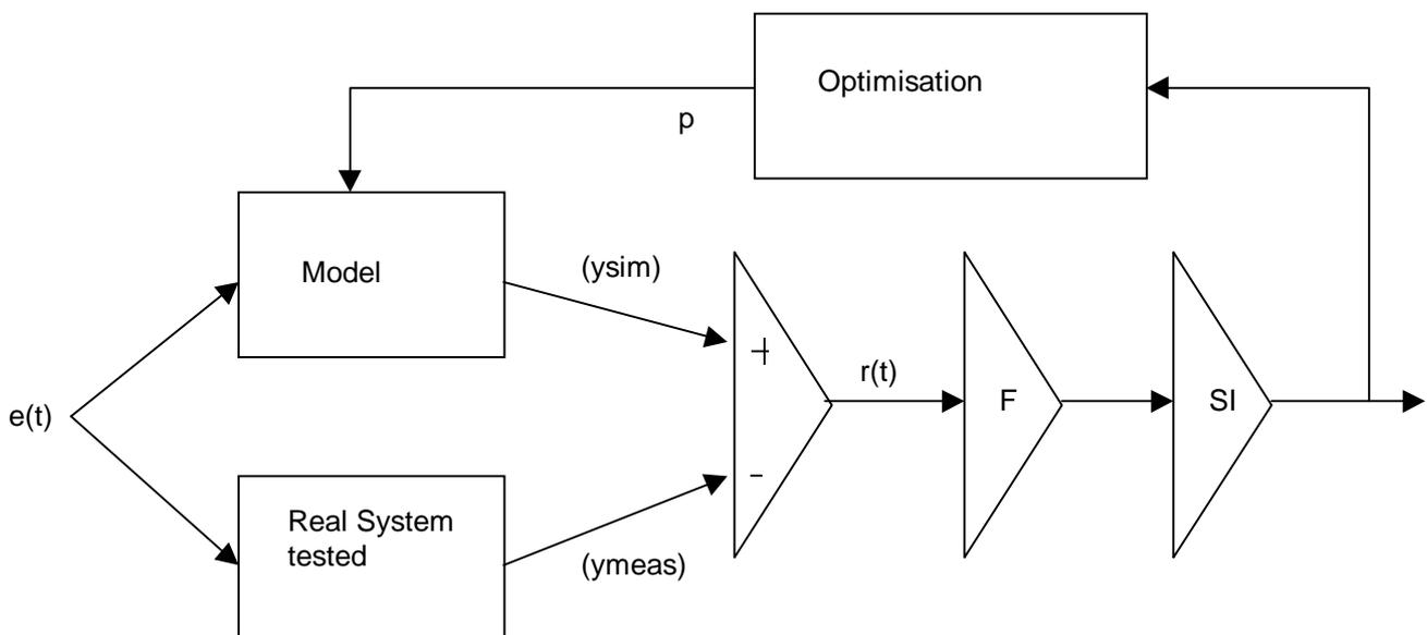
Figure 1. The dynamic fitting procedure (after Spirkl).
