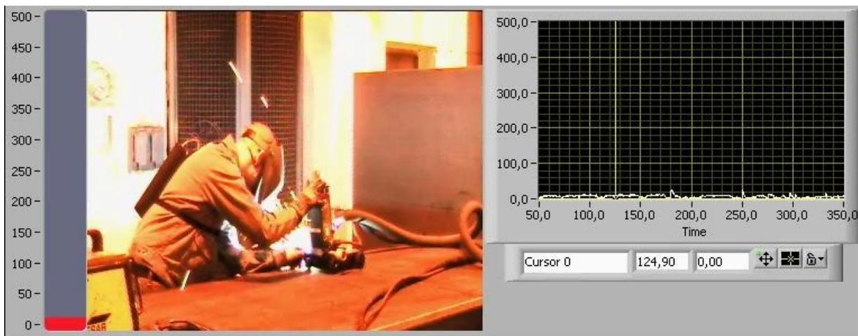
Figure 7. Screen dump from PIMEX recordings comparing exposure to welding smoke (relative values) during welding with a “welding tractor”. The welder is using a provisionally arranged exhaust on the welding pistol.
