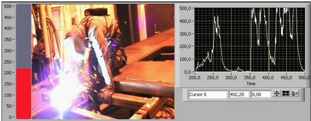
Figure 4. Screen dumps from PIMEX recordings comparing exposure to welding smoke (relative values) during welding with a “welding tractor”. Both welders are doing the same work.
