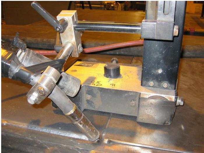
Figure 6. The welding tractor with a provisionally arranged exhaust on the welding pistol.
