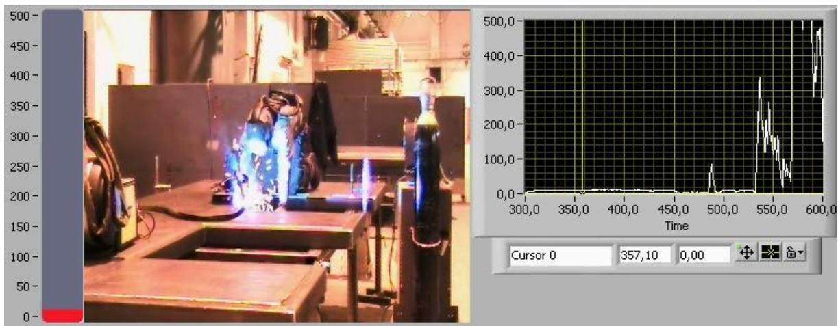
Figure 5. Screen dump from PIMEX recordings comparing exposure to welding smoke (relative values) during welding with a “welding tractor”. The welder is using a fresh air helmet until 530 s (in graph window).
