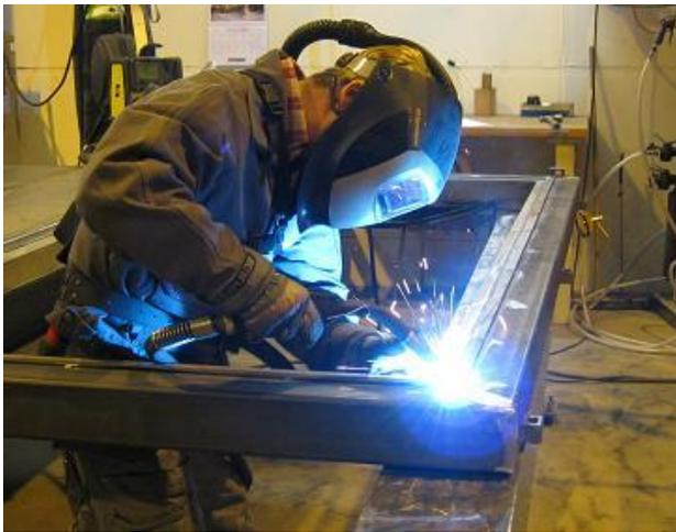
Figure 1. Black sheet welding. The welder is using a helmet with fresh air supply.
