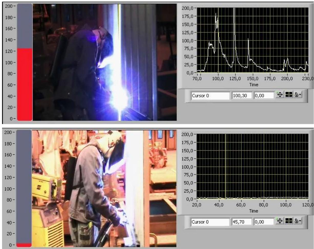
Figure 8. Screen dumps from PIMEX recordings comparing exposure to welding smoke (relative values) during welding in stainless steel. First picture without exhaust on welding pistol. Second with.
