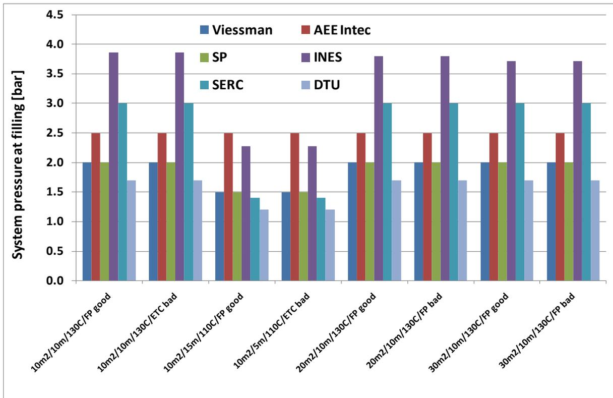
Fig. 5: Comparison of suggested system pressure from the different methods, for the cases defined in table 1.
