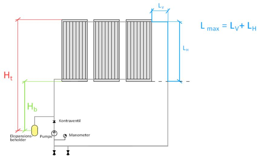
**Fig. 3: Simplified diagram of collector circuit with relevant distances shown.**
