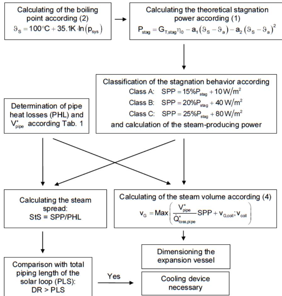
**Fig. 2: Calculation flow chart for calculating the expansion vessel size and whether a cooling device is required in order to protect the expansion vessel. (source: Scheuren and Kirchner [3])**
