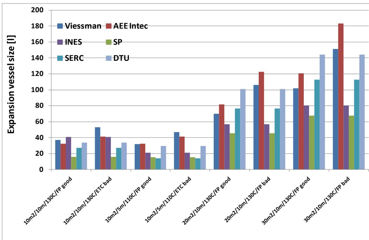
Fig. 6: Comparison of suggested minimum expansion vessel sizes from the different methods, for the cases defined in table 1.
