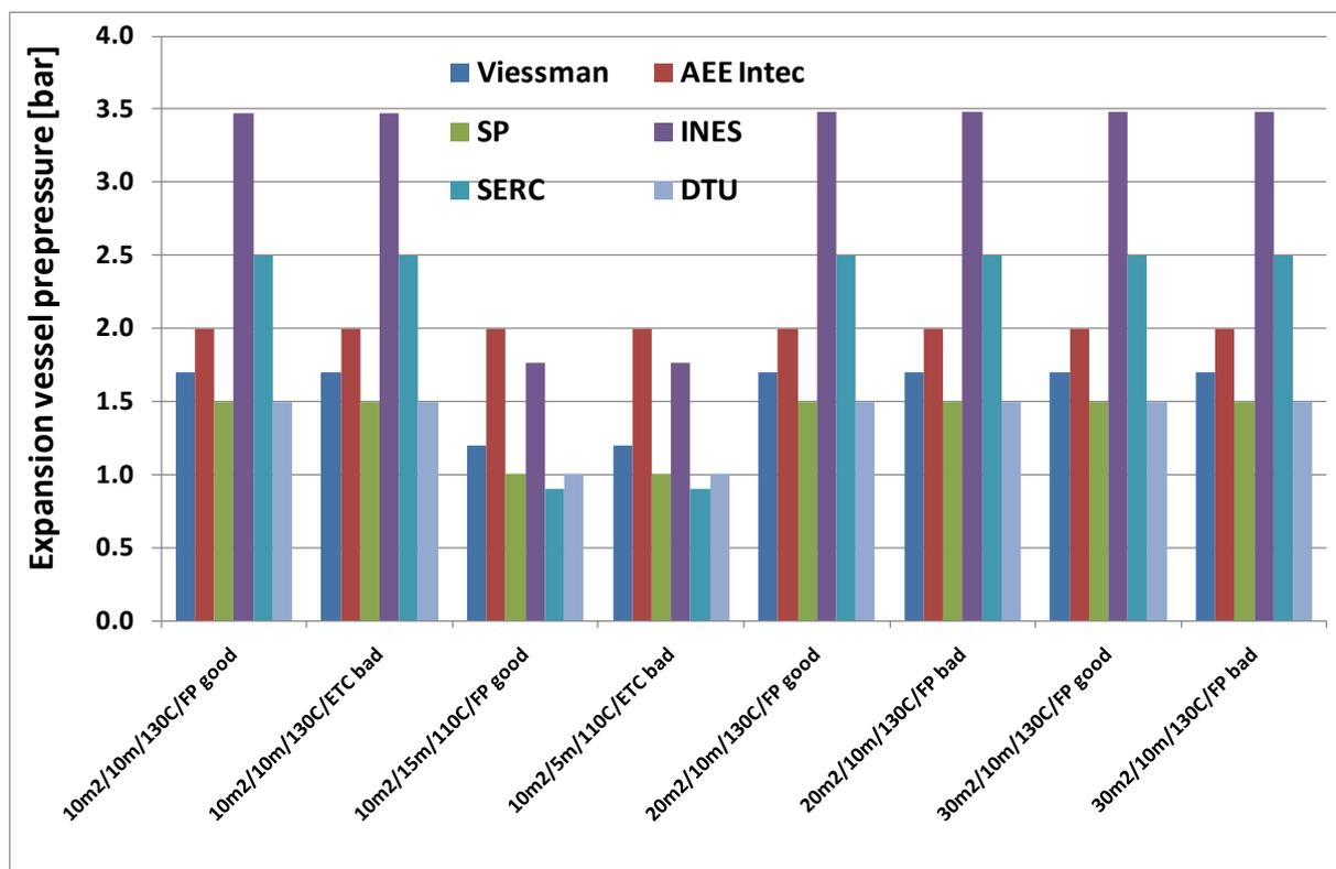
Fig. 4: Comparison of suggested expansion vessel pre-pressure from the different methods, for the cases defined in table 1.
