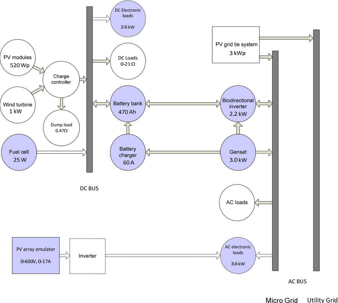
Figure 1: System layout of the PV testing facility.
