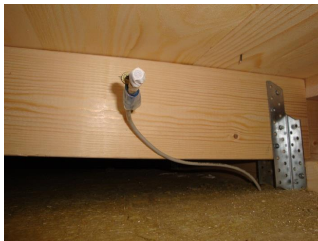
Figure 10. An example of the placing of a sensor, in this case the sensor in the air cavity in the roof.
