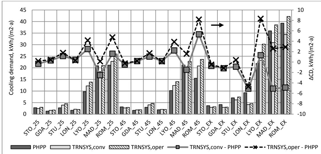
Figure 2. Cooling demand (left axis) and absolute deviation (right axis) between TRNSYS (convective/operative temperature control) and PHPP for the single family house model for all climates and renovation levels.
